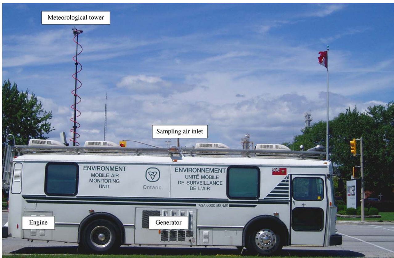
Fig. 1. External view of the mobile TAGA IIe, “Explorer” and retractable meteorological tower.
